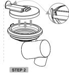
Insert the diaphragm cover into the diaphragm; ensure it aligns the alignment buckle, install it in the correct direction, and fasten it tightly
